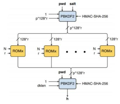
Figure 1: Password conditioning diagram
